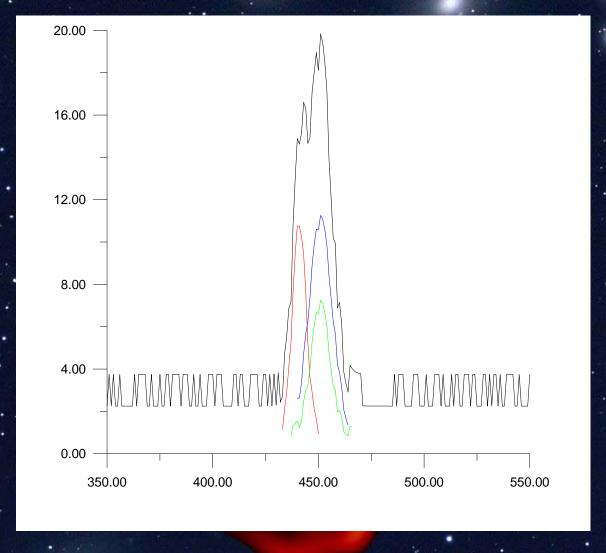
A signal representing a complex spectral line made up of three different components red, blue and green
