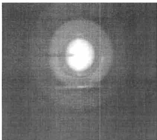
Fig. 2. Photograph of the strata in the air-acetone mixture. P = 5 \text{ Pa} . I = 12 \text{ mA} .
