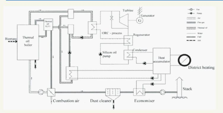
Figure 10 Scheme of the ≈4 MW, CHP facility in Padinska Skela /16/
