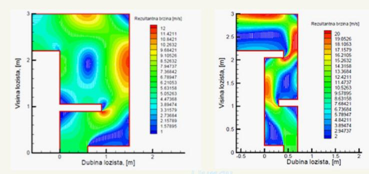
Figure 5 Profiles of the flue gases velocities in two versions of the adiabatic furnace
