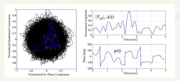
**Figure 6.** Polar plot (left) and time-domain plot of amplitude and phase (right) of a W-CDMA cell-phone signal shows very large swings in amplitude which happen extremely quickly.
