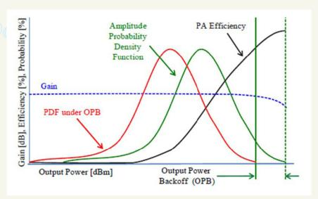
**Figure 7.** Typical PA efficiency and gain behavior over output power. Probability density functions for a high-PAR signal at two average output power levels are overlaid.
