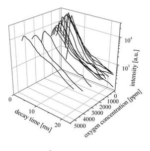
**Fig. 4.** Intensity of nitrogen  $2^{nd}$  positive 0–0 band during the pink afterglow as a function of oxygen concentration.
