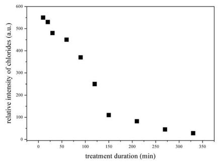
**Fig. 12.** The intensity of chlorides in the corrosion layer of silver coin as a function of treatment duration in the hydrogen discharge. The chloride content was determined using X-ray diffraction analysis.
