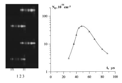
**Fig. 8.** Frames of emission spectrum of erosive plasma flows (left): 1 - line Cu II 456 nm, 2 - line Cu I 459 nm, 3 - line Cu I 465 nm, 4 - line Cu I 515 nm, 5 - line Cu I 522 nm. Temporal dependence of electron concentration (right).
