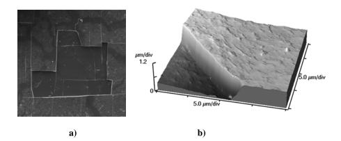
**Fig. 2.** a) SEM micrograph of a typical fracture features and holes on the treated Si (100) surface, image size  $800 \times 800 \ \mu\text{m}^2$ ; b) AFM three-dimensional view of the Si (100) surface morphologies after CPF treatment.
