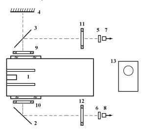
**Fig. 9.** Block diagram of experiments on recording plasma radiation: 1 - discharge device; 2,3 - beam-splitting plate; 4 - flat mirror; 5,6 - optical filters; 7,8 - photodiode; 9-12 - diaphragm; 13 - oscillograph.
