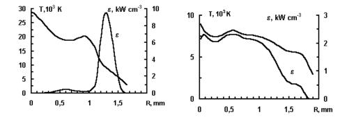
**Fig. 6.** Radial distribution of plasma temperature and emission coefficient for atomic Al I 308.2 nm line in the DP laser plume and z=1 mm at 0.5 (left) and 15 (right)  $\mu$ s from the second pulse action.
