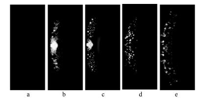
**Fig. 2.** The frame of drop-liquid phase erosion laser jet (diameter of irradiated spot 10 mm) passing time interval  $\Delta t$  after the beginning of acting laser irradiation recession: a)  $\Delta t = 0 \ \mu s$ , b)  $\Delta t = 170 \ \mu s$ , c)  $\Delta t = 260 \ \mu s$ , d)  $\Delta t = 350 \ \mu s$ , e)  $\Delta t = 450 \ \mu s$ .
