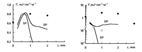
**Fig. 8.** Integrated in time intensity of atomic Al I 308.2 nm (left) and ionic Al II 281.6 nm (right) lines in emission spectra of the laser plume depending on distance z from the sample surface: lines present the modeling results, points show the measurements data for the SP (open circles) and DP (solid circles) modes.
