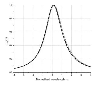
**FIGURE 3.** The  $j_{A,R}(x)$  profiles of neutral atom lines for  $w_e = 2$ ,  $d_e = 0$ , A = 0.075 and different values of: R = 0 (thick line), 0.4 (dashed line) and 0.8 (thin line).
