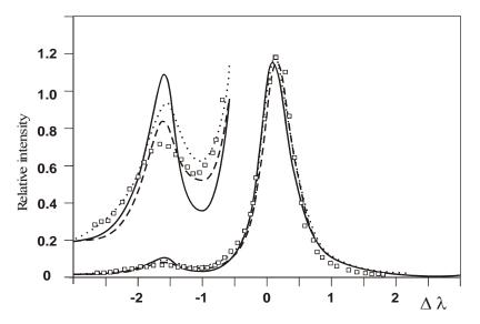
**Fig. 5.** Comparison of measured He I 447.1 nm line shape (squares) with theory: MMM (full), CC (dashed),and BCS (doted line).Plasma parameters:  $N_e = 1 \times 10^{15}$  cm<sup>-3</sup>,  $T_e=18\ 000$  K,  $T_g = 13\ 000$  K. Doppler and instrumental broadening included and all profiles are area normalized.
