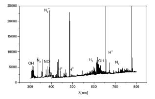
**Fig. 3.** An example of the optical emission spectra obtained during the plasma treatment of archaeological bronze coin.
