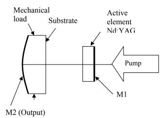
**Fig. 1.** Optical scheme of the Nd:YAG laser with coupled resonators and longitudinal diode pump unit
