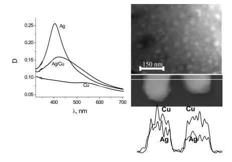
**Fig. 5.** Extinction spectra of silver, copper and bimetallic silver/copper colloids prepared by single-pulse laser ablation (**left**) and SEM images of bimetallic Ag-Cu nanoparticles with distribution of elements along the line of scanning measured by EDX (**right**).
