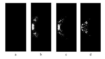
**Fig. 3.** The frame of drop-liquid phase erosion laser jet (diameter of irradiated spot 5 mm) passing time interval  $\Delta t$  after the beginning of acting laser irradiation recession: a)  $\Delta t = 0 \ \mu s$ , b)  $\Delta t = 30 \ \mu s$ , c)  $\Delta t = 250 \ \mu s$ , d)  $\Delta t = 450 \ \mu s$ .
