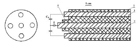
**Fig. 4.** Diagram of the discharge device of the erosive system: 1 - insulator-body, 2 - inner electrode, 3 - roads of outer electrode; I - ignitron,  $C_0$  - energy storage.
