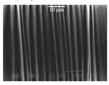
Fig. 6. SEM micrograph of CPF treated silicon surface.
