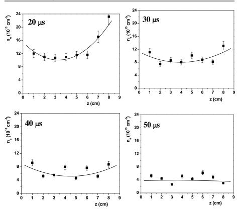
Fig. 2. Electron density axial and temporal dependences in  $N_2 + 5\%$  H<sub>2</sub> at 500 Pa pressure.
