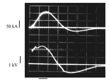
**Fig. 6.** Oscillogram of the discharge current and voltage in the erosive system at  $U_0 = 5 \text{ kV}$ . Bar size is 25  $\mu$ s.
