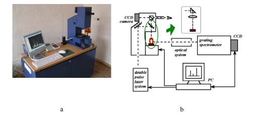
Fig. 1. Laser spectrochemical analyzer: (a) general view and (b) schematic diagram.
