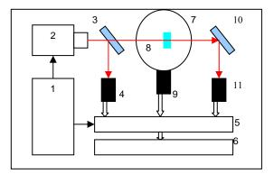
**Fig. 5.** The scheme of experimental equipment for the laser probing. 1 - System of synchronization, 2 - Ruby laser, 3, 10 - Beam splitter, 4, 9, 11 - Photo detectors, 5 - ADC, 6 - Computer, 7 - Integrating sphere, 8 - Sample
