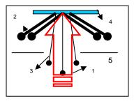
**Fig. 4.** Scheme of the laser erosion mechanism. 1) Acting laser irradiation, 2) The particles formed by hydrodynamic mechanism, 3) The particles formed by the bulk vapor mechanism, 4) Sample, 5) Mask.
