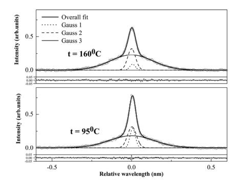
**Fig. 4.** The  $H_{\alpha}$  line profiles recorded along the axis of titanium hollow cathode glow discharge in Ar–H<sub>2</sub> fitted with three Gaussians. Discharge conditions: I=90 mA and p=2 mbar [16].
