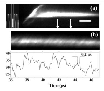
**Fig. 1.** The compression plasma flow intrinsic oscillations: a) Time and space development of CPF from the cathode onwards. Bar size is  $10 \ \mu s$ . b) Enlarged time period indicated by arrows with its light intensity variation represented versus time.
