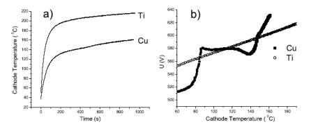
**FIGURE 2.** Measured dependences for two different cathode materials: a) Cathode temperature vs time; b) Discharge voltage vs cathode temperature; Discharge conditions: I = 18 mA, p = 6 mbar of Argon
