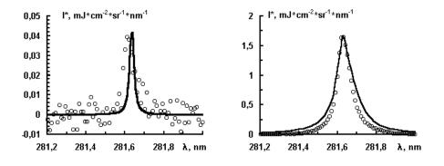
**Fig. 5.** Measured (points) and simulated (lines) profiles of Al II 281.6 nm line in the laser plume emission at SP (left) and DP (right) modes for a side on observation at z=1 mm from the sample surface.
