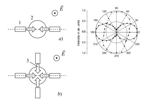
**Fig. 3.** Scheme of transversal pumping of erbium laser AE using two (a) and four (b) LDAs: LDA (1), AE (2), pump radiation (3)
