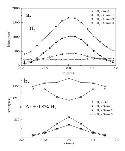
**Fig. 9.** The intensity distribution of the H spectral line and its Gaussian components vs. radial coordinate *r*. Experimental conditions: stainless steel hollow cathode discharge in (a) pure H<sub>2</sub> at p=4 mbar; I=90 mA; U=427V and  $T_{wall}=74^{\circ}C$ ; (b) Ar-H<sub>2</sub> mixture at p=4 mbar; I=90 mA; U=300V and  $T_{wall}=55^{\circ}C$  [28].
