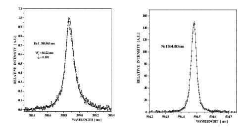
**Fig 2.** a) The recorded He I 388.865 nm line ( $\circ$ ) fitted with  $j_{AR}$  (x) theoretical profile with data taken from [4] for  $N_e = 5.2 \times 10^{22} \text{ m}^{-3}$  and  $T_e = 33000 \text{ K}$  and b) The recorded Ne I 594.483 nm line ( $\circ$ ) fitted with Voigt profile for  $N_e = 4.8 \times 10^{22} \text{ m}^{-3}$  and  $T_e = 33000 \text{ K}$ .
