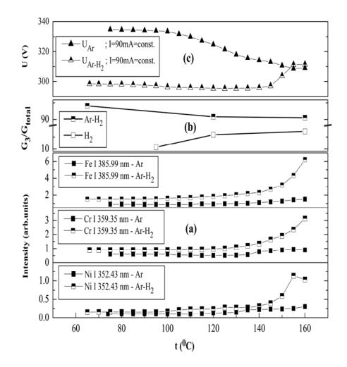
**Fig. 7.** The temperature dependence: of (a) Fe, Cr and Ni resonance lines intensity; (b) contribution of  $G_3/G_{total}$  to the  $H_{\alpha}$  profile in  $H_2$  and in Ar– $H_2$ ; and (c) discharge voltage for constant current of 90 mA in Ar– $H_2$  and in pure Ar [16].
