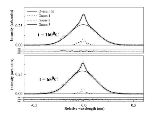
**Fig. 5.** The  $H_{\alpha}$  line profiles recorded along the axis of stainless steel hollow cathode glow discharge in Ar-H<sub>2</sub> fitted with three Gaussians. Discharge conditions: I=90 mA and p=2 mbar [16].
