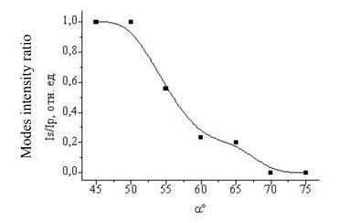
Fig. 2. The dependence of the orthogonally polarized modes intensity ratio on the angle  $\alpha$ .
