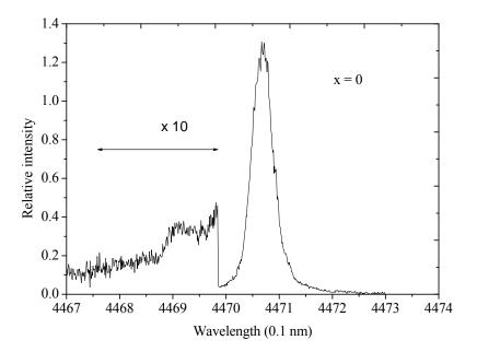
**Fig. 7.** Illustration of line shape recordings with different amplification of the photomultiplier signal. Line emitted from the center of the Mini MIP at height of 1mm from the torch orifice. The flow rate of He through the outer was 0.6 l/min, and He+ 3% H<sub>2</sub> through the inner capillary was 0.2 l/min.
