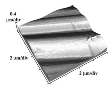
Fig. 4. AFM micrograph of CPF treated Si (100) surface.
