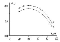
**Fig. 10.** Time variations of spectral absorption constants  $\alpha_{\lambda}$ , at U<sub>0</sub> = 5 kV for spectral intervals: 1) 465-555 nm; 2) 745-1120 nm
