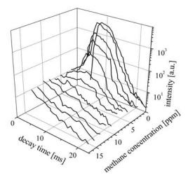
**Fig. 8.** Intensity of nitrogen  $2^{nd}$  positive 0-2 band during the pink afterglow as a function of methane concentration.
