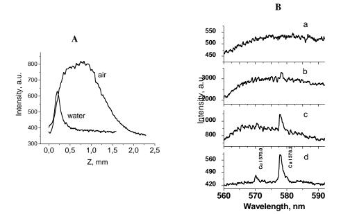
**Fig.2. A** - Intensity profiles in the direction of the normal to the sample surface for emission from the 1064-532 nm double-pulse laser-induced plasma of a copper sample (z = 0 mm), obtained under air and water environment; **B** - fragments of the spectra of the laser-induced plasma of copper sample in case of the 532 nm single (a) and in the 1064-532 nm double-pulse ablation mode for gate delays with respect to the 532 nm laser 200 (b), 400 (c) and 600 ns (d).
