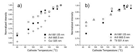
FIGURE 3. Measured line intensities dependance on cathode temperature: a)Discharge with Cu cathode; b) Discharge with Ti cathode; Discharge conditions: I = 18 mA, p = 6 mbar of Argon Difference in sputtering yields for two materials must also be taken into account.
