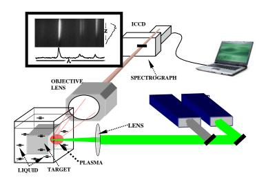
Fig.1. Experimental set-up for time-resolved spectroscopic plasma characterization.
