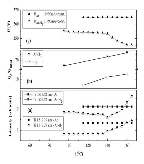
**Fig. 6.** The temperature dependence of: (a) Ti resonance lines intensity; (b) contribution of  $G_3/G_{total}$  to the  $H_{\alpha}$  profile in  $H_2$  and in Ar– $H_2$ ; and (c) discharge voltage for constant current of 90 mA in Ar– $H_2$  and in pure Ar [16].
