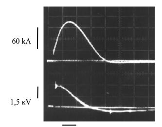
Fig. 2. Oscillogram of the discharge current and voltage in MPC-CG. Bar size is 25  $\mu$ s.
