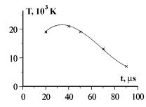
Fig. 11. Time dependence of plasma temperature of a compression erosive flow at  $U_0 = 5 \text{ kV}$ .
