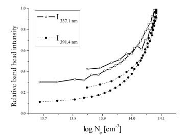
**Fig. 8.** Dependence of the molecular nitrogen band head intensities versus log  $N_e$  for different values of radius in MIP at atmospheric pressure Power input 100 W and flow rate of He 0.7 l/min.
