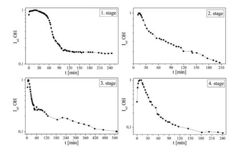
**Fig. 4.** The dependence of the OH band integral intensity as a function of the treatment time during four different stages.
