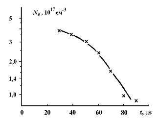
Fig. 7. Temporal dependence of electron concentration in the CPF of MPC.
