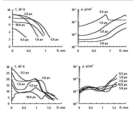
**Fig. 4.** Radial profiles of temperature (left) and density (right) in the laser plumes at the SP (up) and DP (down) modes for a distance z=1 mm from the sample surface at different time intervals from the laser pulse action (shown in micro-seconds).
