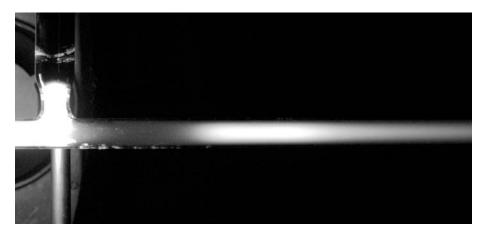
Fig. 1. Pink afterglow in pure nitrogen DC post-discharge.
