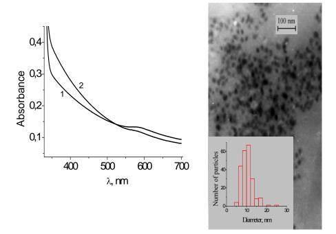
**Fig. 4.** Extinction spectra of copper nanoparticles prepared in acetone: (1) by the repetitive (10Hz) 1064 nm single-pulse laser ablation for 5min; (2) by the double-pulse laser ablation (10  $\mu$ s separation between the 1064nm and 532 nm pulses) (**left**) and TEM image with corresponding size distribution histogram of Cu nanoparticles prepared in single pulse regime in acetone (**right**).
