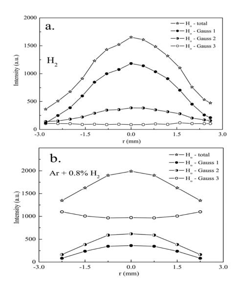
**Fig. 10**. The intensity distribution of the H spectral line and its Gaussian components vs. radial coordinate. Experimental conditions: titanium hollow cathode discharge in (a) pure H<sub>2</sub> at p=4 mbar; I=90 mA; U=424V and  $T_{wall}=75^{O}C$ ; (b) Ar-H<sub>2</sub> mixture at p=4 mbar; I=90 mA; U=338V and  $T_{wall}=75^{O}C$  [28].
