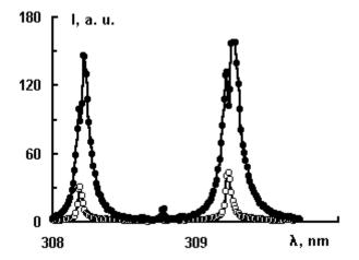
**Fig. 2.** Emission spectra of the laser-induced Al plasma at SP (open circles) and DP (solid circles) modes recorded 1 mm above the sample surface (one can see atomic lines Al I 308.2 and Al I 309.3 nm).
