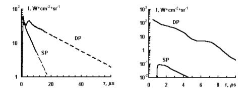
**Fig. 7.** Total intensity of atomic Al I 308.2 nm (left) and ionic Al II 281.6 nm (right) spectral lines in the SP and DP laser plume emission at z=1 mm depending on time from the laser pulse action. Dashed line shows the data extrapolation.
