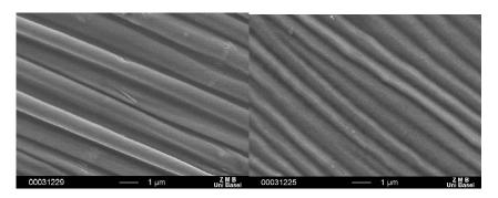
Fig. 5. SEM micrographs of highly oriented periodical structures on treated silicon surface.
