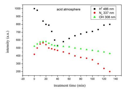
**Fig. 8.** The dependence of the spectral band integral intensity as a function of the treatment time during the plasma model samples treatment. The corrosion layer was made in acid atmosphere.
