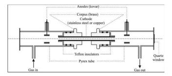
Fig 1. The hollow cathode discharge tube [13].
