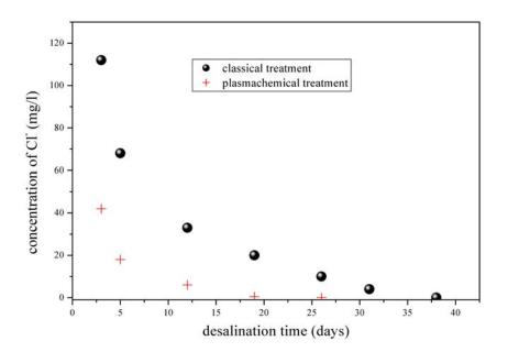
**Fig. 5.** The dependence of the concentration of Cl<sup>-</sup> as a function of the desalination time in the case of classical and plasmachemical treatment of iron artefacts. The concentration was determined by titrimetric (mercurimetric) method.
