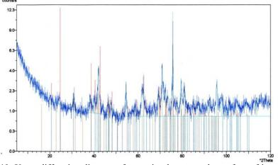
**Fig. 10.** X-ray diffraction diagram of corrosion layers on the surface of iron object before plasma treatment. The main peaks correspond to the geothite FeO(OH), lepidocrocite  $Fe_2O_3 H_2O$  and FeOCl
