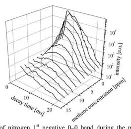
**Fig. 9.** Intensity of nitrogen  $1^{st}$  negative 0-0 band during the pink afterglow as a function of methane concentration.
