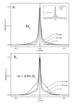
**Fig. 8.** Typical H<sub>a</sub> profiles recorded at different radial positions in: (a) stainless steel hollow cathode; upper right corner depicts the H<sub>a</sub> line shape at radial position r=2.8 mm fitted with three Gaussians; and (b) titanium hollow cathode. Discharge conditions: (a) pure H<sub>2</sub> at p=4 mbar; I=90 mA; U=427V and  $T_{wall}=74^{\circ}C$ ; (b) Ar-H<sub>2</sub> mixture at p=4 mbar; I=90 mA; U=338V and  $T_{wall}=75^{\circ}C$  [28].
