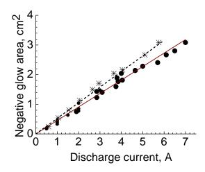
**Fig. 3.** Dependence of the area of the negative glow S on discharge current for the APGD in helium: closed circles – copper cathode, snowflakes – stainless steel cathode.
