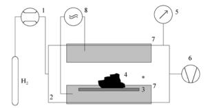
**Fig. 1.** 1 – mass flow controller; 2 – Pyrex glass reactor (length 100 cm, inner diameter 10 cm); 3 – Pyrex artifact holder; 4 – the treated archaeological artifact; 5 – baratron gauge; 6 – rotary oil pump; 7 – outer cylindrical copper electrodes; 8 – RF power supply; \* – point of spectroscopic measurements.
