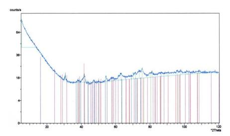
**Fig. 11.** X-ray diffraction diagram of corrosion layers on the surface of iron object after 60 minutes of the plasma treatment. The main peaks correspond to the magnethite,  $Fe_3O_4$ , hematite  $Fe_2O_3$  and calcium iron oxide  $CaFe_3O_5$ .
