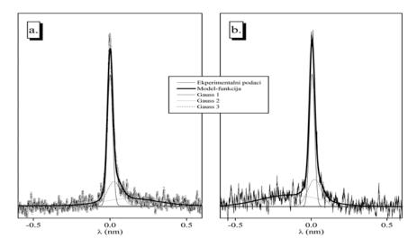
**Fig. 3.** Typical  $H_{\alpha}$  line shapes recorded end-on from low pressure high-voltage discharge (He-H<sub>2</sub>) mixture; stainless steel cathode) and fitted with three gaussians: (a) front anode and (b) rear anode. Discharge conditions: p=1mbar, U=1030V,  $I\approx5$ mA. [13]
