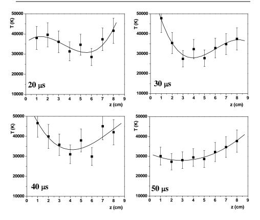
Fig 1. Electron temperature axial and temporal dependences in  $N_2$  + 5% $H_2$  at 500 Pa pressure.
