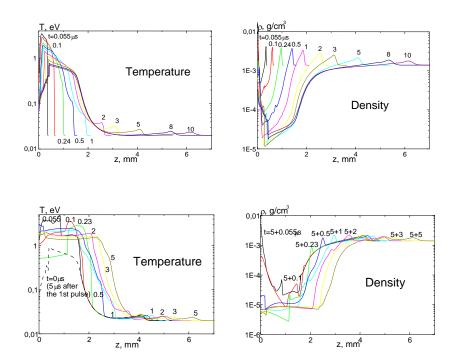
**Fig. 3.** Axial distribution of plasma temperature and density in the laser plumes at SP (up) and DP (down) modes at different time intervals from the laser pulse action (shown in micro-seconds).
