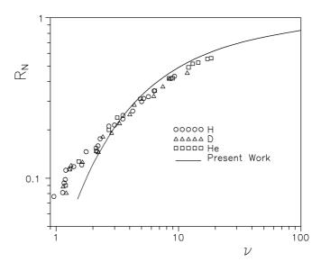
Figure 2: Particle reflection coefficient for light ions incident normally on heavy targets. Comparison of the present work with the computer simulation data of Vicanek et. al.
