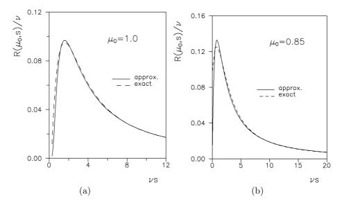
Figure 1: Path-length distributions of backscattered ions calculated for (a) perpendicular incidence and (b) oblique incidence.
