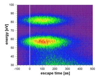
Figure 2: Energy vs. run time of electrons emitted from the surface.
