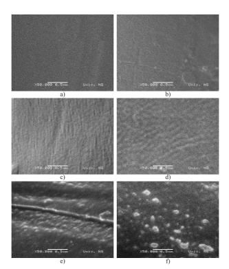
Figure 1: SEM images of a) untreated PES; b) untreated PA; c) corona treated PES; d) corona treated PA; e) corona treated PES loaded with silver NPs and f) corona treated PA loaded with silver NPs.
