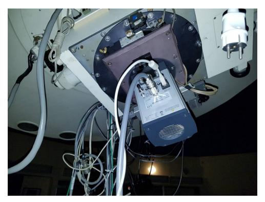
**Figure 3:** The 2 m telescope (NAO Rozhen) with new CCD camera Andor iKon-L.
