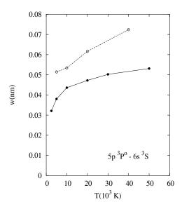
**Figure 1:** Stark widths due to electron impacts for Cd I 5p  ${}^{3}P^{o}$  - 6s  ${}^{3}S$  (494.13 nm) spectral multiplet as a function of temperature. Values of Dimitrijević and Konjević (1983) are presented by white points, and values of Simić, Dimitrijević and Sahal-Bréchot (present results) by black points.
