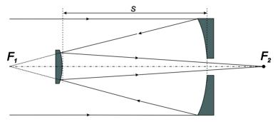
Figure 1: Scheme of a two-mirror system:  $F_1$  is the primary mirror focus,  $F_2$  is the effective focus and s is the distance between the two mirrors.
