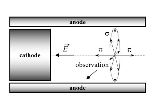
The central part of the modified Grimm GDS and the schematics of  $\pi$  and  $\sigma$  light polarization. By rotating the linear polarizer axis for 90 degrees, the  $\pi$  or  $\sigma$  polarization is selected.
