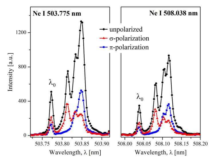
3-component unpolarized profile [1] and polarized profiles with 3  $\sigma$  and 2  $\pi$  components, recorded at ~15 kV/cm electric field strength.  $\lambda_0$  denotes an unshifted zero-field line.
