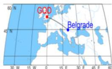
Fig. 1 Great Circle Paths (GCPs) of subionospherically propagating VLF radio signals recorded at Belgrade site.
