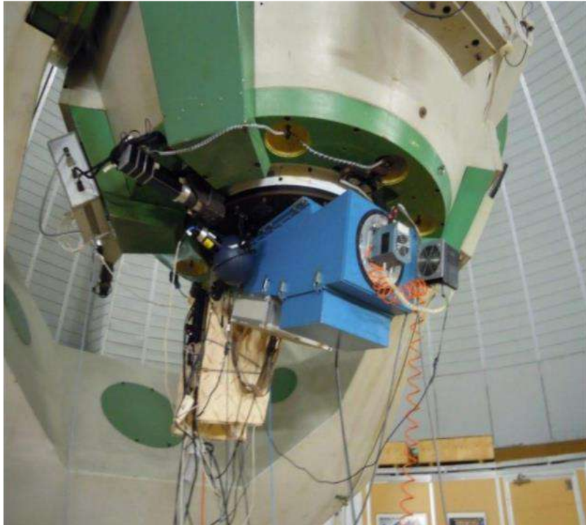
Copernico 1.82-m telescope Italy, Asiago AFOSC (double WP + 100Å filters)
