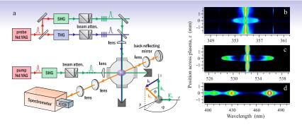
Experimental setup (a) and typical images of TS spectra at 355 nm (b) and 532 nm (c) and of plasma emission spectra (d). [Dzierżęga et al., 2021]
