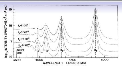
Wall-stabilized arc [Wiese et al., 1972]. The last observed discrete line is clearly a function of the plasma density.
