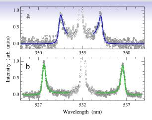
Typical TS spectra recorded on the plasma axis for two probe lasers of  $355\,\mathrm{nm}$  (a) and  $532\,\mathrm{nm}$  (b). Solid lines: the best fit with the electron spectral density function
